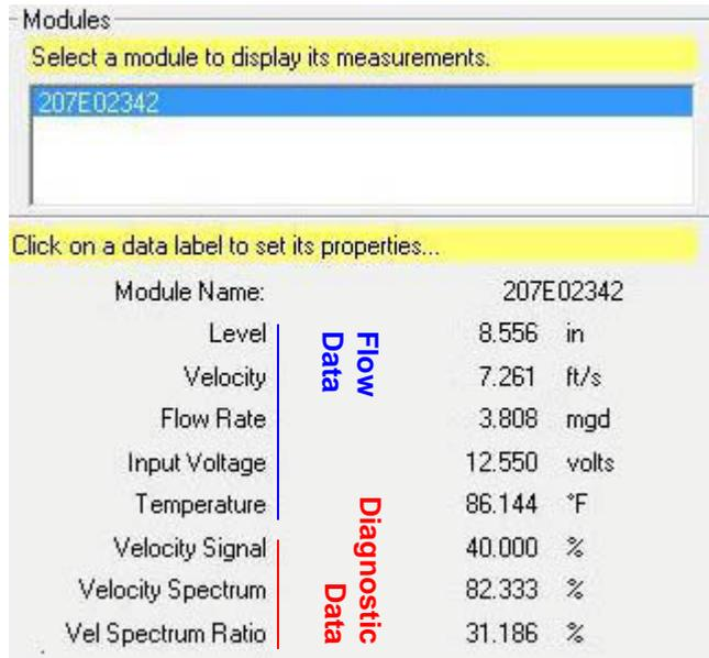
**FIGURE 2. Text report displaying real-time flow and diagnostic data**
