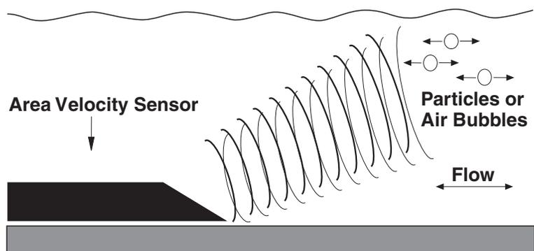
**FIGURE 1. AV Sensor operation**
