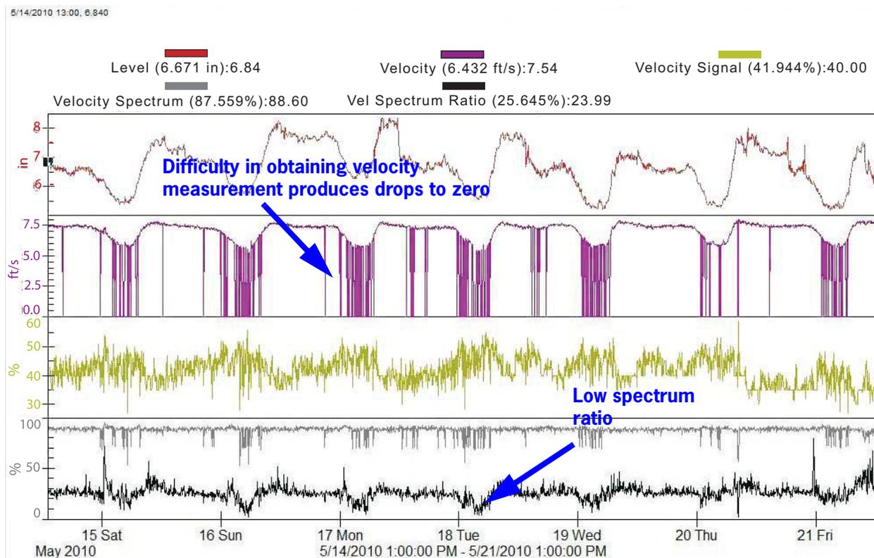
FIGURE 5. Diagnosis of velocity dropouts using spectrum ratio
